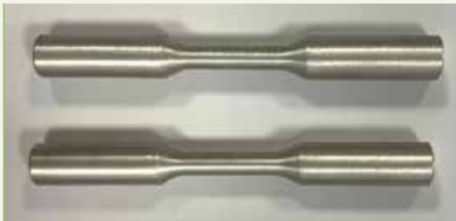
Test pieces ready for testing (6 mm gauge diameter)
