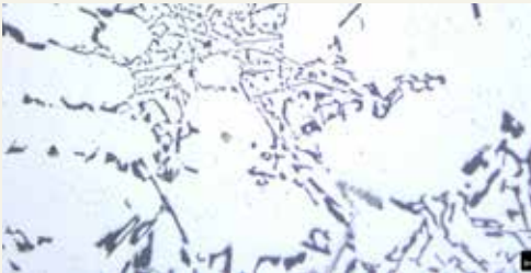
Alloy microstructure without Sr (500× magnification)
