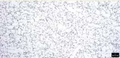
Alloy microstructure in T6 temper (200× magnification)
