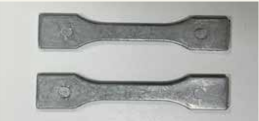
Test pieces ready for testing (3 mm thick)
